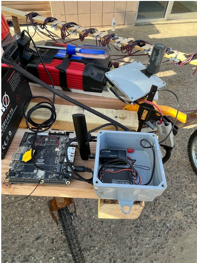
Figure 5. Early scanner, approximately May–June 2023: distance sensors, compute board, battery and GPS. [P1, P9]
